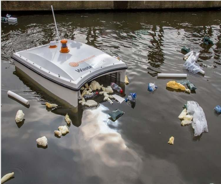
Aqua Drone : trash cleaner and environmental data collector
